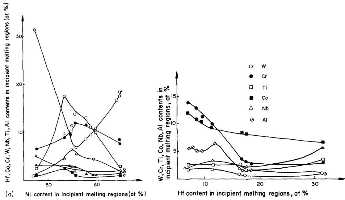
Figure 3 Variation of elements in the incipient melting regions, as a function of (a) nickel content, (b) hafnium content. (○) hafnium, (●) cobalt, (□) chromium, (■) tungsten, (△) niobium, (▲) titanium, (⊗) aluminium.
