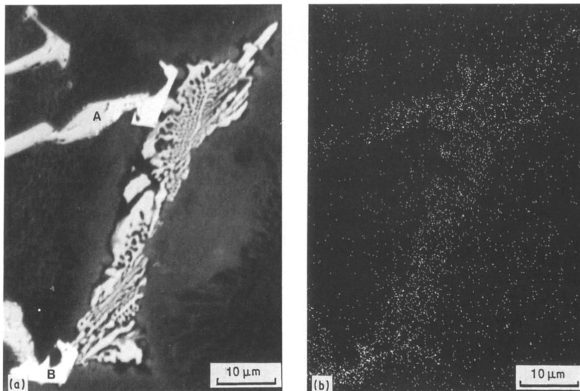
Figure 2 An incipient melting region in the DS200 + Hf alloy. (a) Cellular- and columnar-like morphology. A and B are carbide particles connected to the incipient melting region: (b) hafnium, (c) nickel, (d) titanium, (e) chromium.
